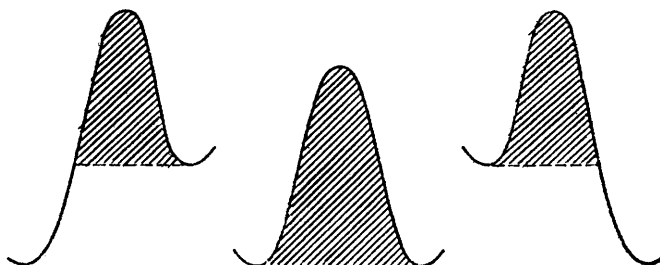
Figure 4 Tunnelling regions (shaded areas) as a function of barrier symmetry (Reproduced by permission from 'The Proton in Chemistry', 2nd edn., Chapman and Hall, London, 1974)
